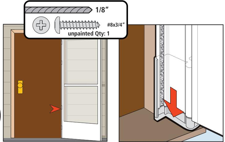
**5D** Slide rail extender into sill. Loosen inside jamb screw as needed.
